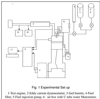
7-TDC marker and speed sensor, 8- Data acquisition system and loading device , 9-Exhaust gas calorimeter, 10-Smoke meter, 11-four gas analyzer, 12-computer, 13 & 14 Fuel tanks
